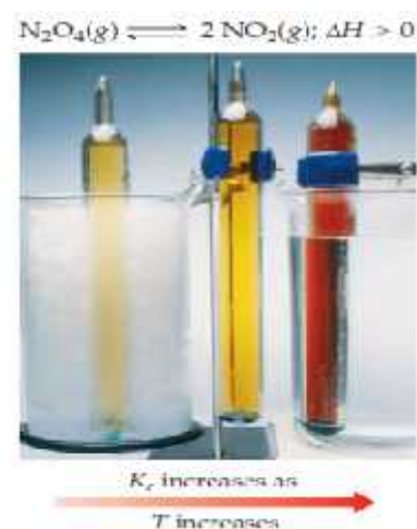
Figure 3. Sample tubes containing an equilibrium mixture of Nice water (left), at room temperature (center), and immersed in hot water (right) (Murry & Fay, 2012)
